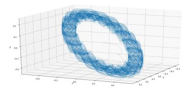
Figure: A forced oscillation (obtained in the perturbed Chua's circuit) with a numerical estimate  $\overline{\dim}_B \mathcal{M}_u \approx 2.5$  and upper estimate  $\leq 2.5$  [M. A., V. R., A. R., 2019]. The upper estimate is given by formula (14) for  $\alpha = 2/3$ , m = 2,  $\beta = 0$  and  $\theta = 1$ .
